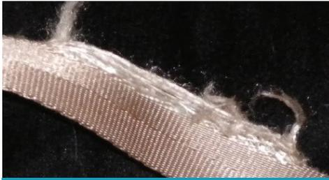
Frequent use and sun exposure can damage seat components and weaken plastic (eg. fraying, cracking and white stress marks on plastic)
